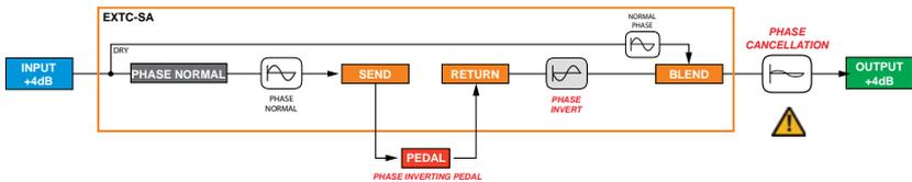
The PHASE INVERT switch plays an important role by ensuring both the dry and wet signals are in phase. The next diagram shows how the PHASE INVERT switch reverses the signal polarity before it gets to the offending pedal. Pedal "B" gets tricked into re-inverting the signal back to normal phase.
