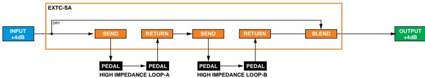
Although simple in principle, the key to the EXTC-SA's performance is how quietly it does the task. This is achieved by employing full sized discrete electronic components, class-A circuitry and transformer isolation to help eliminate the hum and buzz that is common with pedals and guitars. The other cool 'trick' inside the EXTC-SA is the blend control. This mixes the original dry signal with the newly introduced effects created by the pedals.
