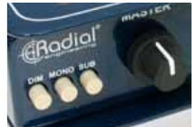
As with the monitors and sub outputs, you can set the DIM attenuation level using the set & forget DIM LEVEL ADJUSTMENT control on the top panel. The attenuated level is usually set quite low so that you can easily communicate over the playback volume. The DIM is sometimes used by engineers who like to mix at low levels to reduce ear fatigue. Being able to precisely set the DIM volume makes it easy to go back to familiar listening levels with a push of a button.
