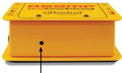
GROUND LIFT OUT-2: Use a small screwdriver to access the ground lift switch for OUT-2. Set inward to lift the ground (factory default) or outward to connect ground.
