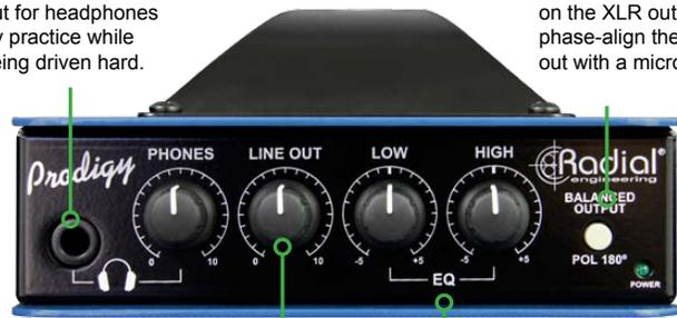
**LINE OUT** - Variable control to adjust the level going to the unbalanced 1/4" JDX outputs.
