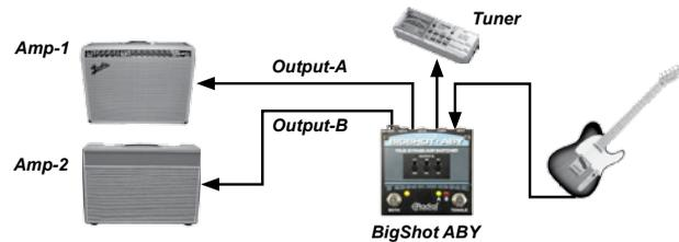
2. **At this point it is important to read the caution statement on the back cover and ensure all your equipment is properly grounded.** If your equipment meets all electrical safety requirements, you may connect the amplifiers to an AC power outlet.
