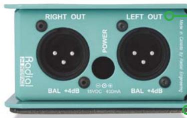
**STEREO OUTPUT** balanced line-level low-z XLR outs drive long cable with +4dB signal level.
