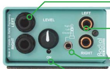
**STEREO HI-Z INPUTS** accept unbalanced electronic instruments and line-level signal.
