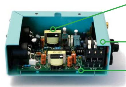
**HIGH PERFORMANCE** transformer for distortion-free signal transfer and 100% isolation from ground loop hum.
