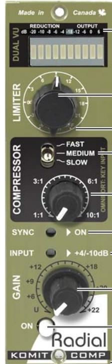
**DUAL BALLISTIC VU** - 10-segment LED ladder is divided into two meters. The left side indicates gain reduction while the right conveys the output level.
