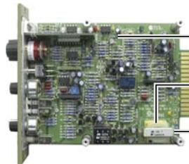
**12 POSITION SWITCH**: Military-grade Grayhill switch features gold contacts and steel shaft for years of trouble-free performance.
