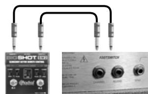
Guitar cables used with separate footswitch jacks.
