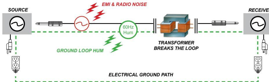
*The image above shows an audio source and a destination with a common electrical ground. As the audio also has a ground, these combine to create a ground loop. The transformer and ground lift work together to eliminate the ground loop and potential noise.*
