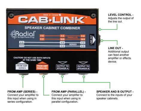
**Combine cabinets in series configuration** Connect two 8 Ohm speaker cabinets in series to use with a 16 Ohm amplifier output. **Combine cabinets in parallel configuration** Connect two 8 Ohm speaker cabinets in parallel and run both from a single 4 Ohm output on your amplifier. Use the line out to feed another amplifier Run a second amplifier from the line out for a wet/dry setup. Fine tune the output with the level control.
