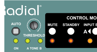
Threshold control sets the sensitivity of the auto-switch detector
