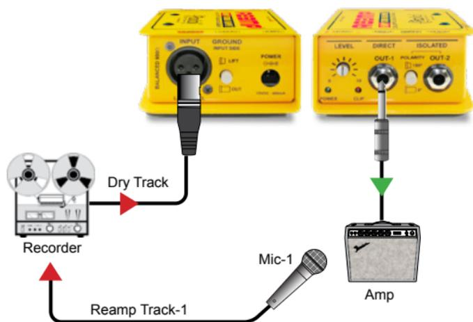
Reamping the dry track and recording new tracks.
