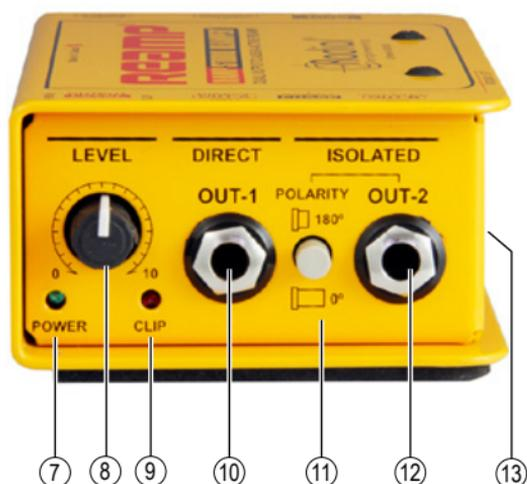
8. **LEVEL CONTROL:** The output LEVEL control sets the volume level going to the guitar amplifiers. This potentiometer is recessed to prevent accidental change and is adjusted using a guitar pick or flat-head screwdriver.
