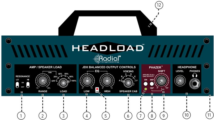
1. **RESONANCE:** Increases the high and low frequency resonance. Used to compensate for weak bass and/or treble response when listening at low volume levels.
