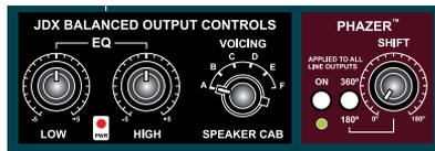
The Phazer can reinforce the fundamental frequency making the combination of the JDX and mic sound thicker and richer than either do on their own. You can also experiment with the Phazer and create special effects. Use your ear while adjusting the SHIFT control and choose the setting that sounds best.
