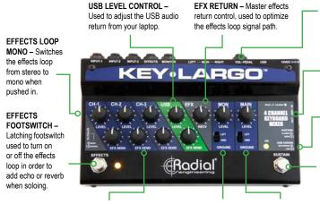
LEVEL CONTROL (CH1, 2, 3) – Used to adjust the input levels of your three analog keyboards.
