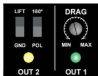
*The Headlight will only switch between the outputs that have an amp connected. If only OUT-1 is connected the SELECT switch will have no effect.*
