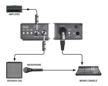
Try moving the microphone around the room to find the sweet spot where the fundamental frequencies or harmonics line up to create a satisfying tone from the two sources. You can also send the JDX 48 signal to the left speaker and the mic signal to the right speaker to create a stereo effect.
