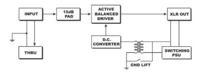
After the paralleled input and thru jacks the signal passes through a switchable 15dB PAD which allows the Pro48 to handle virtually any audio device from passive pickups to high output instruments without overloading.
