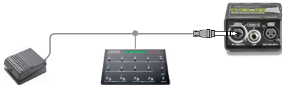
Simple footswitches and contact-closure devices like MIDI controllers use 1/4" cables to connect to the Relay Xo.
