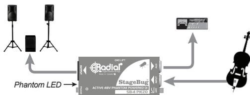
As an active direct box, the SB-4 requires 48V phantom power from the console to make it work. Phantom power is a standard feature that is readily available on all consoles and must be turned on. Once activated, the LED on the SB-4 will illuminate to let you know that it is powered and ready for use.
