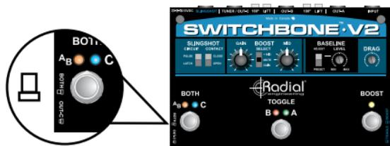
When the BOTH/OUT-C set & forget switch is in the OUT position, the Switchbone V2 is configured like a typical ABY switcher. In this mode, the tuner output is always on. When the BOTH/OUT-C switch is pushed inwards, it changes the BOTH function to add OUT-C so that no signal will be present on TUNER/OUT-C unless the footswitch is depressed. When used for a third amp, you should check for noise and phase following the steps detailed above. Always use Amp-A as the reference for phase.
