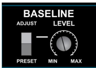
The Baseline™ buffers the signal, lowering noise by lowering the impedance. High impedance circuits are much more susceptible to picking up stray magnetic fields and radio frequencies. Once the signal is buffered, you can essentially drive the cable a much longer distance when using a quality coaxial cable.
