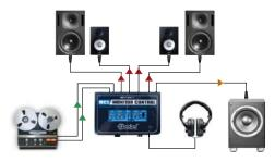
The MC3 Monitor Control connects from the output of your recording system and feeds two sets of monitors, a sub-woofer, ear buds and three headphones!
