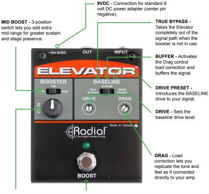
GAIN - Delivers up to 18dB of clean gain for soloing and taking total control on the
