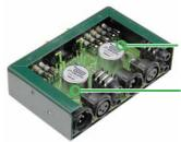
**Jensen -** Nickel core transformer for distortion-free signal transfer and 100% isolation.
