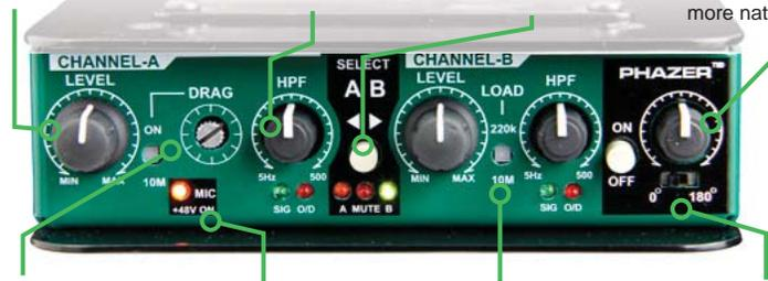
**DRAG** - Load correction used to set the desired impedance on the pickup for the most natural tone.
