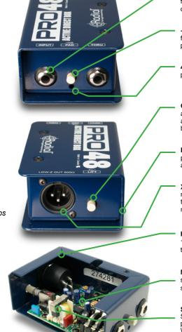
**INPUT & THRU -** ¼" input connects from instrument, the parallel ¼" THRU connects to an on-stage amplifier.
