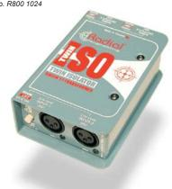
The Radial Twin-Iso is a balanced 2 channel, +4dB line-level isolator that has been specifically developed for professional touring systems as a means to eliminate hum and buzz caused by ground loops when interfacing various equipment such as two consoles, remote towers and drive racks.
