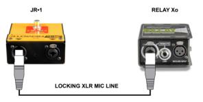
Another advantage is that XLR cables can be daisy-chained together to make a longer cable. This means you won't have to depend on a specific custom built cable to connect your remote device.
