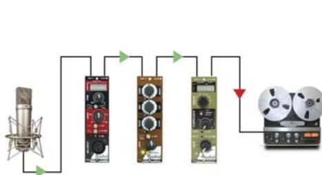
**USING THE Q3 IN A CHANNEL STRIP**
