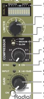
DUAL BALLISTIC VU - 10-segment LED ladder is divided into two meters. The left side indicates gain reduction while the right conveys the output level.
