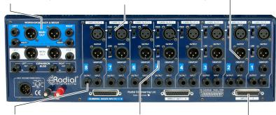
MODULE I/O: Follows original format and adds parallel ¼" TRS jacks for cross-patching between modules.
