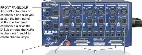
EXTERNAL AC SUPPLY: 1600mA of shared current for power-hungry tube modules.
