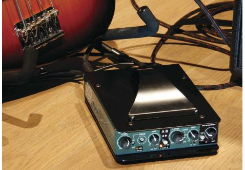
The actual phantom power switch is on the side of the box, along with a button to blend channels A and B, and an Aux out/direct switch that lets you introduce an isolation transformer into a stage amp output signal path to reduce ground hum or buzz.
