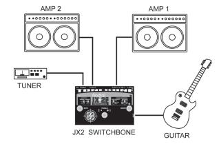
To reduce opportunity for shock hazard or damage to the JX2 or connected equipment, plug the ½" connectors into the amplifiers first and then to the JX2. This is especially important when using old amplifiers that do not have 3-prong plugs as the possibility exists to touch the chassis ground with the connector plug tip when the plug is inserted into the jack.
