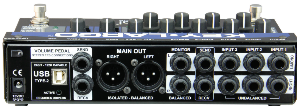
Fig. 1. At a glance, the rear panel tells you the balanced/unbalanced status of ins and outs, that the volume pedal send/return is stereo-capable, and that you need drivers for USB (though only on Windows, natch). No manual-diving needed!
