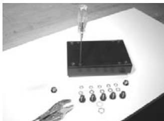
Knobs off, nuts & washers off, side jack nuts & washers off, now removing screws.
