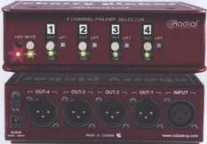
Since the Cherry Picker is a "straight wire" line device, its also possible to connect it to the output of your favorite mic or instrument preamp and then send its outputs to four different compressors or eqs to quickly audition choices there as well.
