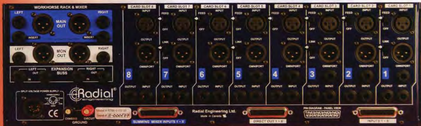
The rear panel hosts a number of I/O options, including a D-sub input for the summing amp, and direct outputs from each module.
