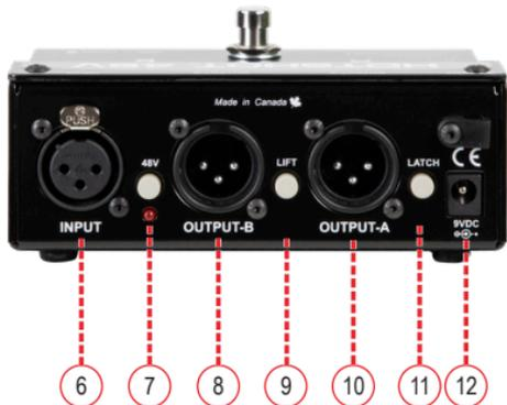
6. **INPUT:** Balanced XLR input for connection to a microphone.
