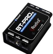
The BT-Pro V2 is a Bluetooth-enabled direct box that connects wirelessly to smartphones, tablets, and other mobile devices and provides a pair of balanced analog audio outputs to feed a PA system. Each BT-Pro V2 has a unique identifier, allowing multiple units to be used within the same building. The latest model of the BT-Pro V2 can also be powered via 48V phantom from a mixing console.
