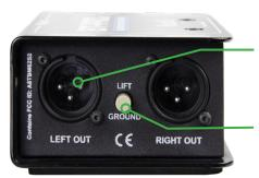
XLR OUT - Standard male XLR outputs provide balanced analog audio at mic or line-level to feed a PA system. The BT-Pro can be powered remotely by providing 48V phantom power to these outputs.
