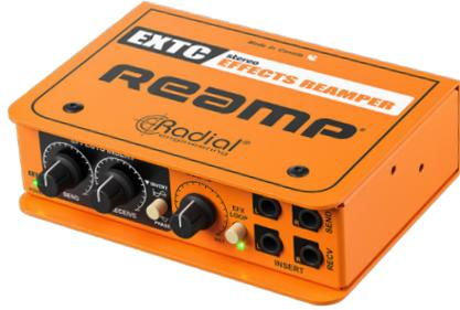
The EXTC Stereo is a creative studio tool that gives you the ability to play any pre-recorded audio track through stereo guitar effects pedals, using the process known as Reamping™ to utilize your pedal collection in new and exciting ways.
