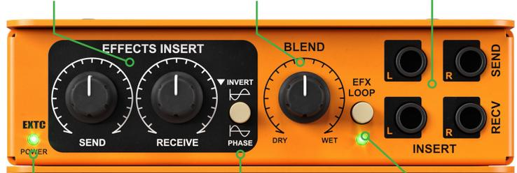
**POWER LED** - Illuminates to indicate the EXTC Stereo is connected to power.
