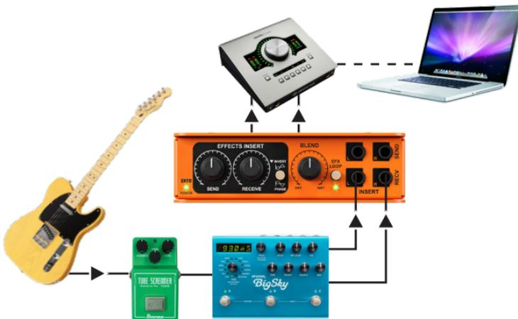
Using the EXTC Stereo for direct recording
