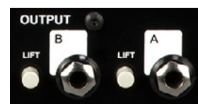
The amp outputs and lift switches
