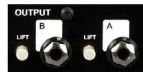
*The amp outputs and lift switches*
