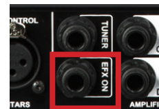
The EFX ON remote input jack
