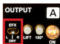
The EFX Assign switch for Amp-A
