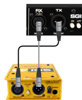
The balanced XLR connections from the SGI-44 to the JX44.
