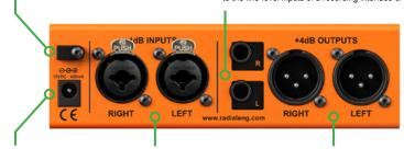
**PSU IN:** Connection for the included 15V 400mA power supply.
