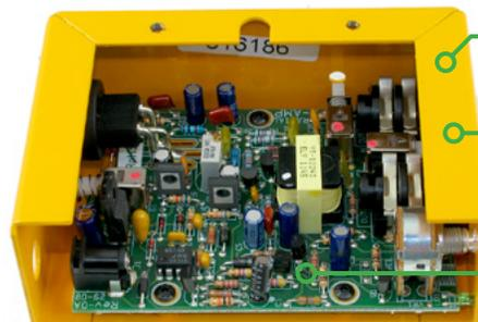
**HEAVY-DUTY WELDED I-BEAM** - Enclosure of 14 gauge steel makes it impossible to torque the PC board. Eliminates cold solder joints.
