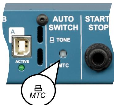
To feed MTC (MIDI Time Code) to the Auto-Switch inputs, set the rear panel AUTO-SWITCH input selector to the 'in' position. Then setup your Digital Audio Workstation (DAW) to feed MTC to the SW8-USB. This will require you to enable the MTC generate/transmit function in your DAW, and to select the SW8-USB as the output destination. Refer to the user guide for your DAW for details on where these settings are located (ProTools MTC settings shown below).
