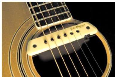
Magnetic pickup in acoustic guitar sound hole.
