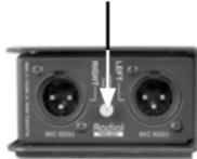
The second ground lift is simply labeled **LIFT** and is located on the input panel. This switch allows the right channel ground to be lifted separately from the left channel and is intended for dual mono applications where one source device needs a ground path through the ProAV2 while the other may not. Note that the **GROUND** switch supersedes the **LIFT** switch and disconnects the ground path for both channels regardless of the position of the **LIFT** switch.
