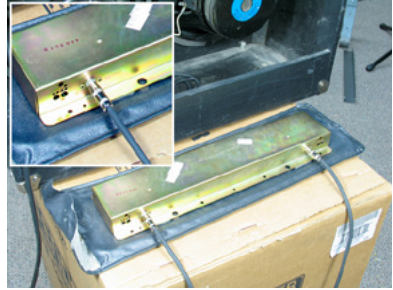
If the tank cables are hard-wired into the chassis you can expose the tank and connect directly to it.
